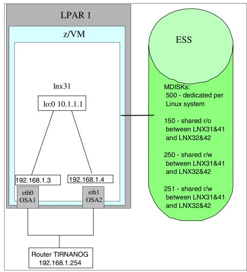
Figure 11 Configuration for OSA adapter failure
