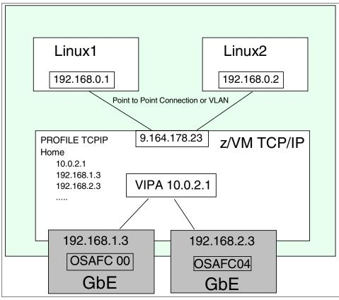
Figure 5 VIPA configuration with z/VM as TCP/IP router and Linux guest systems
