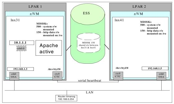
Figure 12 Test setup Apache failover
