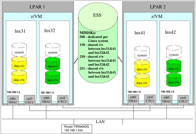
Figure 10 Hardware setup for the test environment
