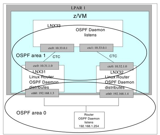
Figure 16 Configuration of Linux router failover test
