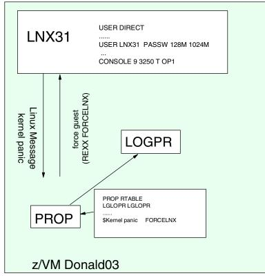
Figure 3 PROP configuration and message flow
