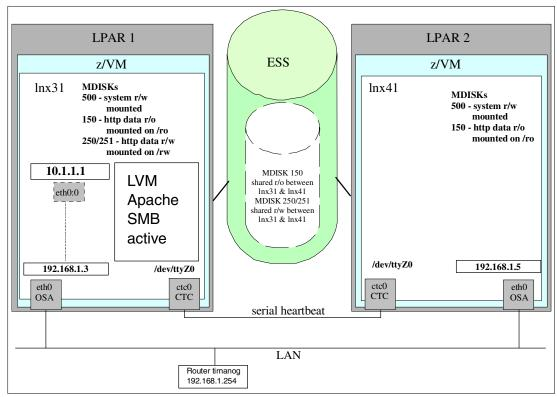
Figure 14 Setup for SAMBA server failover
